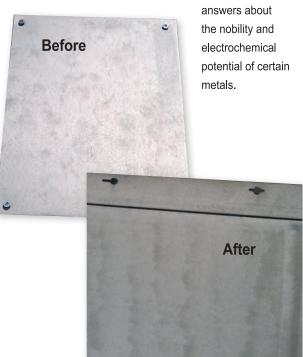
In most environments and applications, FreedomGray Satin T-Z Alloy™ will not stain other materials below them. However, drip edges and overhangs should still be designed to minimize water staining.
