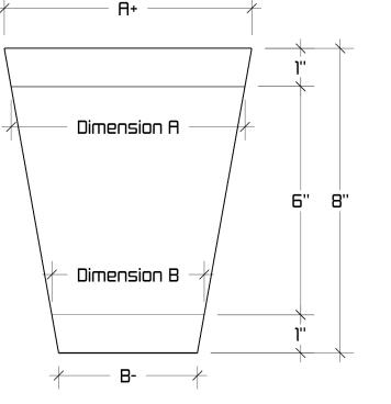
The example to the left shows a 6" (A) to 4" (B) adapter. That dimension change is achieved over 6" in height for all adapters, however, all are extended by 2" (1" in each direction). This allows the adapter to receive a downspout and be inserted into another (receive a 6" and be inserted into a 4" in this example).
