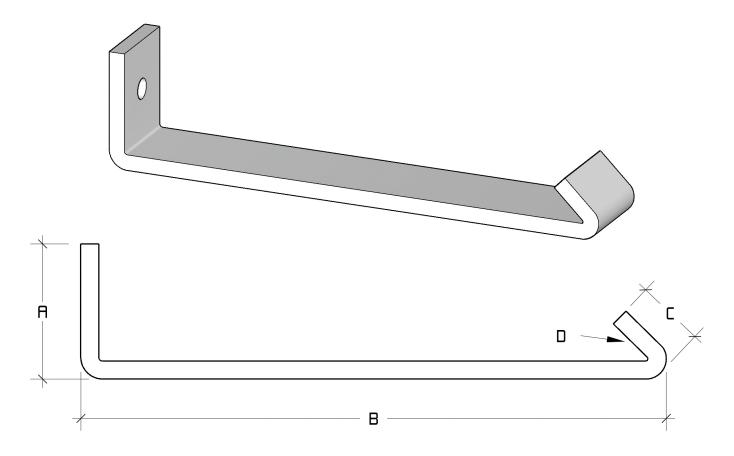
Available in 3/16" aluminum and copper bar stock as well as 1/8" stainless steel. Fits most manufacturer's large Box Gutters and K-Style Gutters. Please check dimensions. Works with all K&M's standard Box Gutters and K-Style Gutters.
